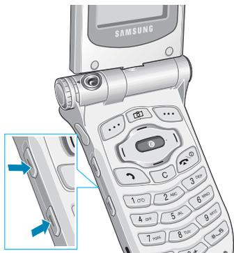
In Idle Mode, you can also adjust the keypad tone volume using these keys.
