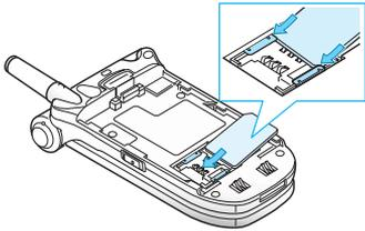
**Note:** When you need to remove the SIM card, slide it, as shown, and take it out of the socket.
