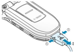
**Note:** You must unplug the adapter before removing the battery from the phone during charging; otherwise, the phone could be damaged.
